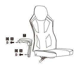
STEP 6 / 步骤六 Aim at the top of gas lift and the hole of mechanism, then put the chair body down.
